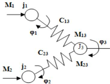
$$\begin{cases} \varphi_1 = \frac{M_1 - M_{13}}{j_1 p^2}; \\ \varphi_2 = \frac{M_2 - M_{23}}{j_2 p^2}; \\ M_{13} = C_{13}(\varphi_1 - \varphi_3); \\ M_{13} = C_{23}(\varphi_2 - \varphi_3); \\ \varphi_3 = \frac{M_{13} + M_{23}}{j_3 p^2}; \end{cases}$$
