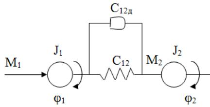
$$\begin{cases} \varphi_1 = \frac{M_1 - M_2}{J_1 p^2} \\ \varphi_2 = \frac{M_2}{J_2 p^2} \\ M_2 = C_{12}(\varphi_1 - \varphi_2) + C'_{12}(\omega_1 - \omega_2) \end{cases}$$
